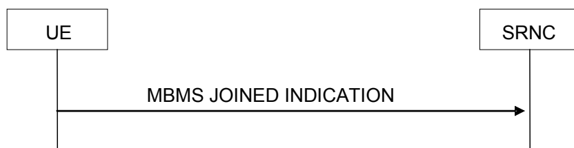
Figure 8.3.6: MBMS joined indication signalling flow
