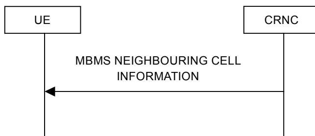
Figure 8.3.5: MBMS Neighbouring Cell Information signalling flow
