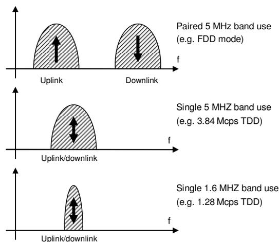
Figure 5 – WCDMA Paired Spectrum and TD-SCDMA Unpaired Spectrum [18]
