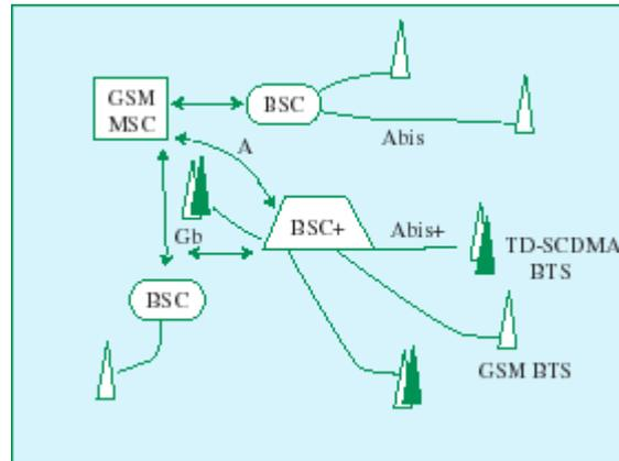
**Figure 3 - Schematic Diagram of TD-SCDMA System. Used in GSM Network, Providing 3G Services [15]**
