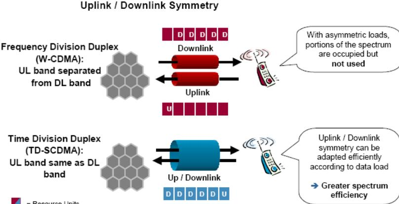
**Figure 9 - Uplink and Downlink Differences in TD-SCDMA and WCDMA [4]**
