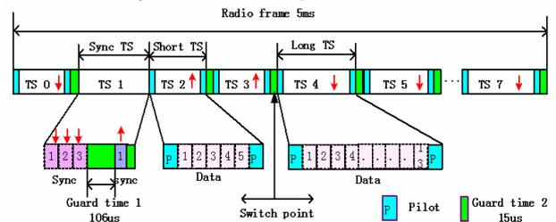
Figure 5. Frame structure of FuTURE B3G TDD
