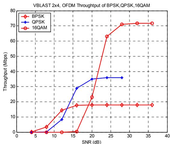
Figure 6. The throughput of the VBLAST OFDM system
