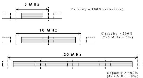
Figure 7. Capacity Vs. scalable bandwidth
