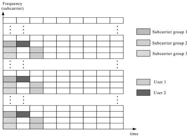
Figure 3. The resource structure of OFDMA/TDMA system
