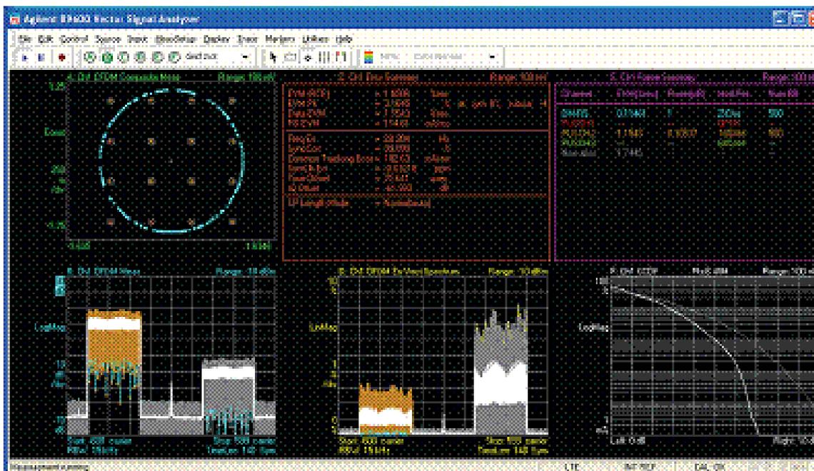
**Figure 8** Analysis of a 16QAM SC-FDMA signal
