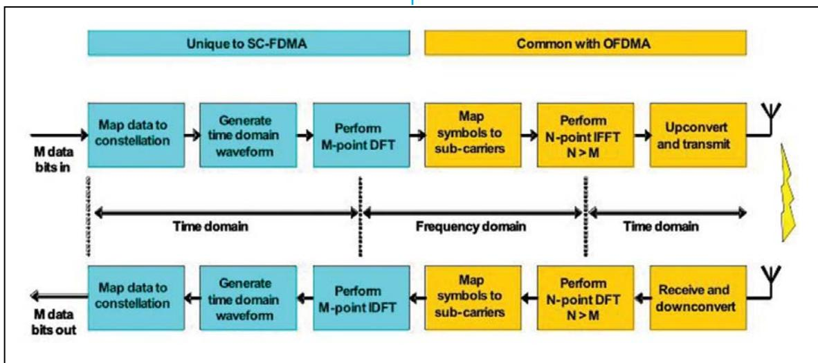
**Figure 5** Simplified model of SC-FDMA generation and reception
