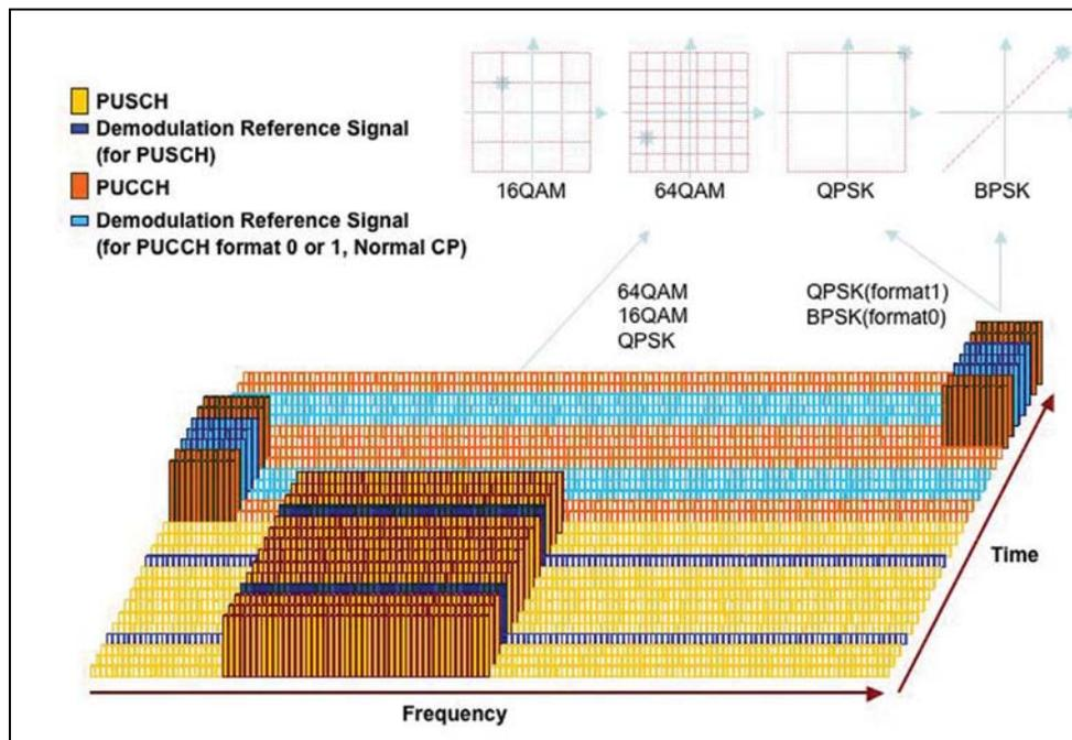
Figure 7 Frame Structure 1 for the uplink showing one subframe vs. frequency
