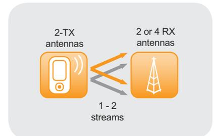
Figure 7. Uplink dual antenna transmission for HSUPA.
