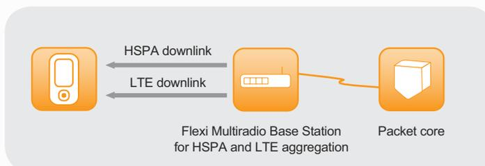
Figure 4. HSPA and LTE carrier aggregation.
