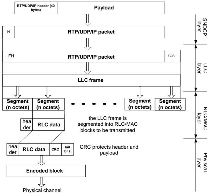
Figure 2 – Segmentation and channel coding for streaming or “download & play”
