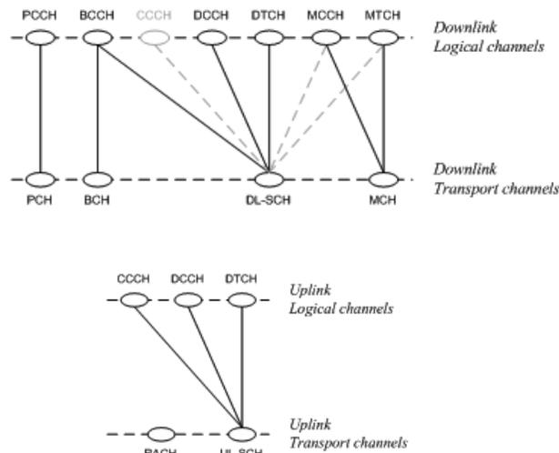
Figure 8: Logical to transport channel mapping [4]
