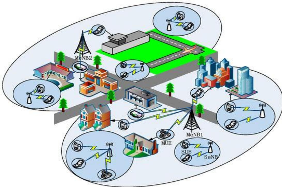
Figure 2. HetNet: small cells offloading traffic. Source: M. Li, P. Chen, and S. Gao, "Cooperative Game-Based Energy Efficiency Management over Ultra-Dense Wireless Cellular Networks," *Sensors*, vol. 16, 2016.
